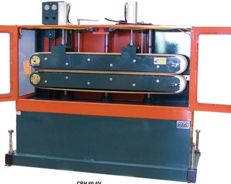
CBH 60-6V 6" x 60" contact area Vector motor and pneumatically-activated top conveyor
